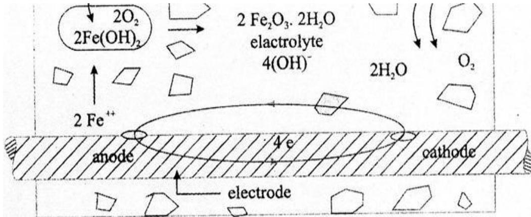
Simplified model representing corrosion mechanism
