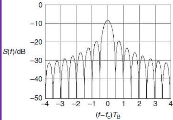
Normalized power-spectral density of quadrature-phase shift keying.
