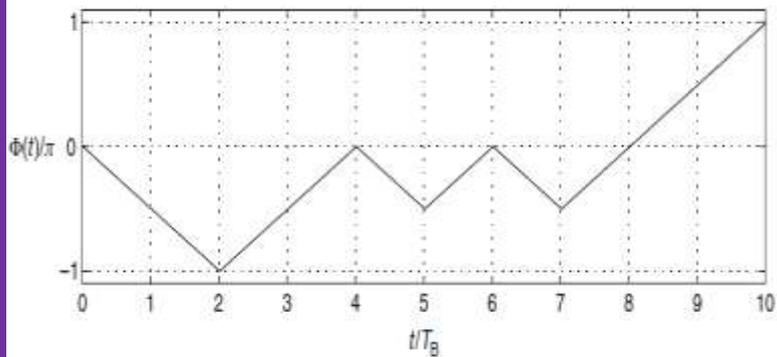
Figure 11.32 Phase pulse and phase as function of time for minimum shift keying signal.
