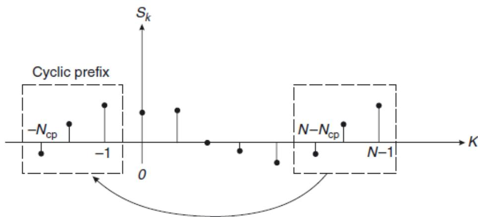
This operation removes the first part of the received signal (of duration  $T_{cp}$ ) from the detection process; the matched filtering of the remainder can be realized as an FFT operation. The signal at the output of the matched filter is thus convolution of the transmit signal with the channel impulse response and the receive filter:
