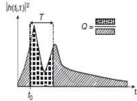
Figure 6.10 Definition of window parameters.
