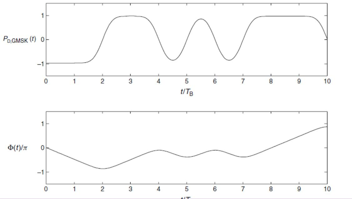
Pulse sequence and phase of Gaussian minimum shift keying signal
