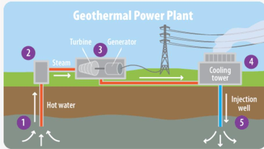
1. Hot water is pumped from deep underground through a well under high pressure.
