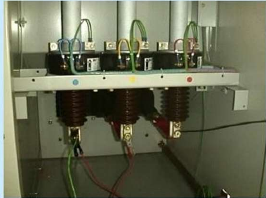
High voltage lightning impulse test on 11 kV switchgear (MAHKOTA MANUFACTURING SDN BHD)
