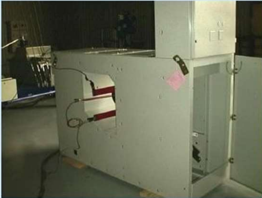
High voltage lightning impulse test on 11 kV switchgear (MAHKOTA MANUFACTURING SDN BHD)
