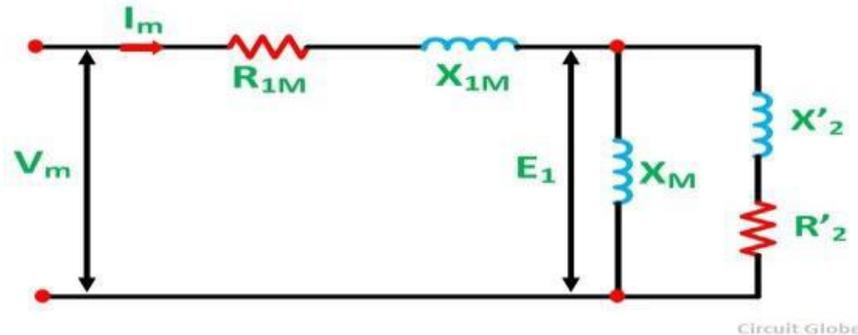
The simplified equivalent circuit of a single phase induction motor with only its main winding energized is shown in the figure below.
