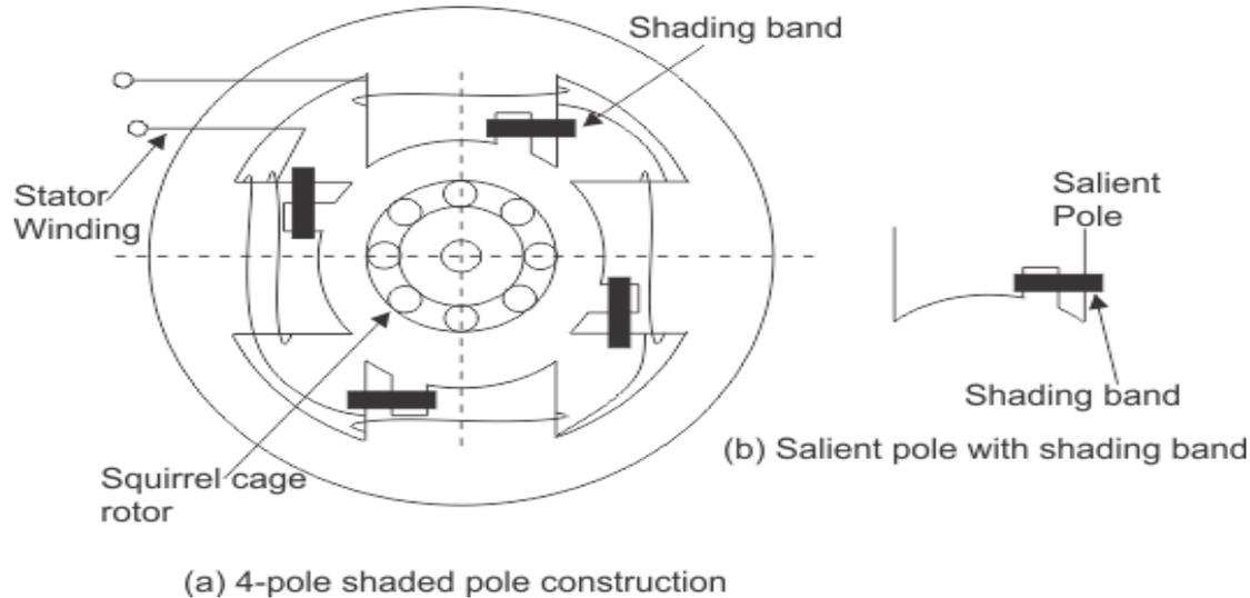
The stator of the **shaded pole single phase induction motor** has salient or projected poles. These poles are shaded by copper band or ring which is inductive in nature. The poles are divided into two unequal halves. The smaller portion carries the copper band and is called as shaded portion of the pole.
